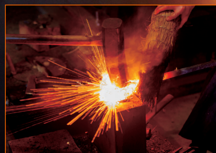
The sparks that fly during forging are from impurities burning off. The steel is folded and hammered up to 15 times, resulting in 32,768 (2 to the 15th power) layers.
